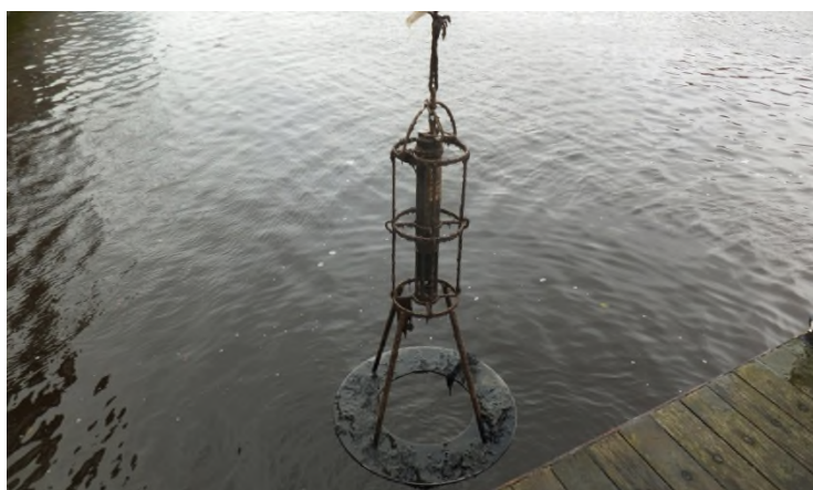
Figure 2: ICE buoy river bed deployment.
