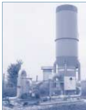
Figure 2.6 | Example of a forced air enclosed flare
