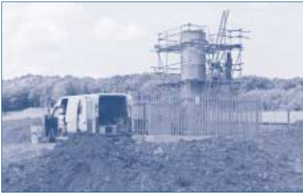
Figure 5.1 | In-stack enclosed flare monitoring with grid of probes (right) for emissions monitoring
