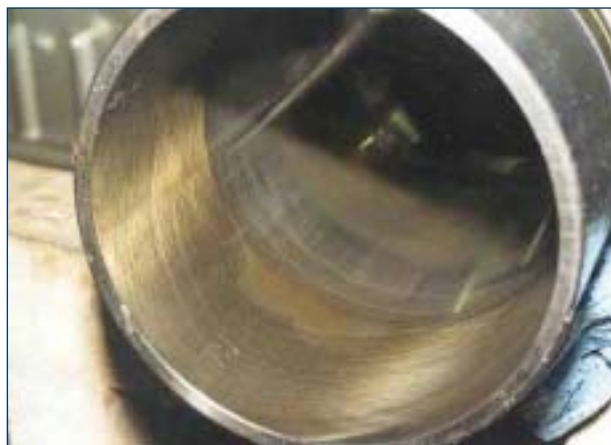
Figure 2.1 | Golden lacquer of siloxane build-up evident on cylinder liner
