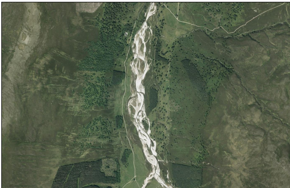
Figure 6: Aerial image of a typical braided and wandering section of the River Feshie near Glenfeshie Lodge. Note the multiple channels and large areas of exposed sediment in the channel which show that frequent erosion, transport and deposition occurs. The active channel is up to 200m wide in places.
