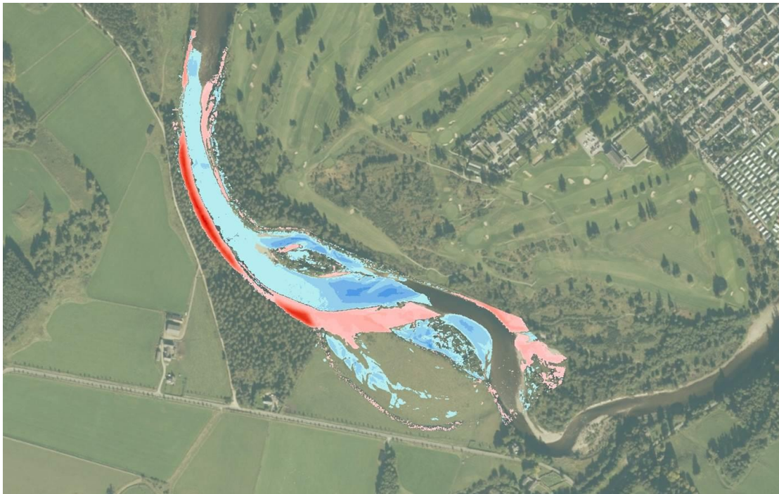
Figure 54: Aerial image of the “Red Brae” area overlaid with comparison of LiDAR between 2011 and 2016. Colours as per Figure 53. © Getmapping
