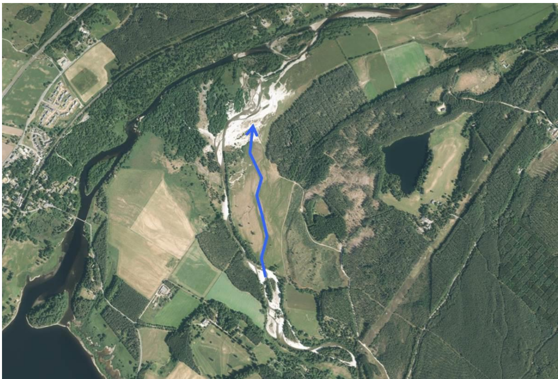
Figure 21: Aerial image of reach overlaid with option to realign channel to a lower part of the alluvial fan utilizing an old channel. © Getmapping
