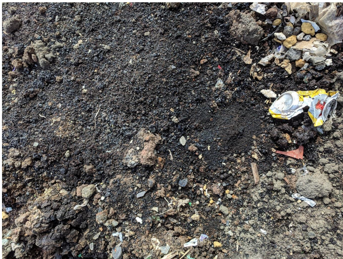
Figure 18 - Ash waste and other waste materials exposed at surface at Tarbolton Landfill
