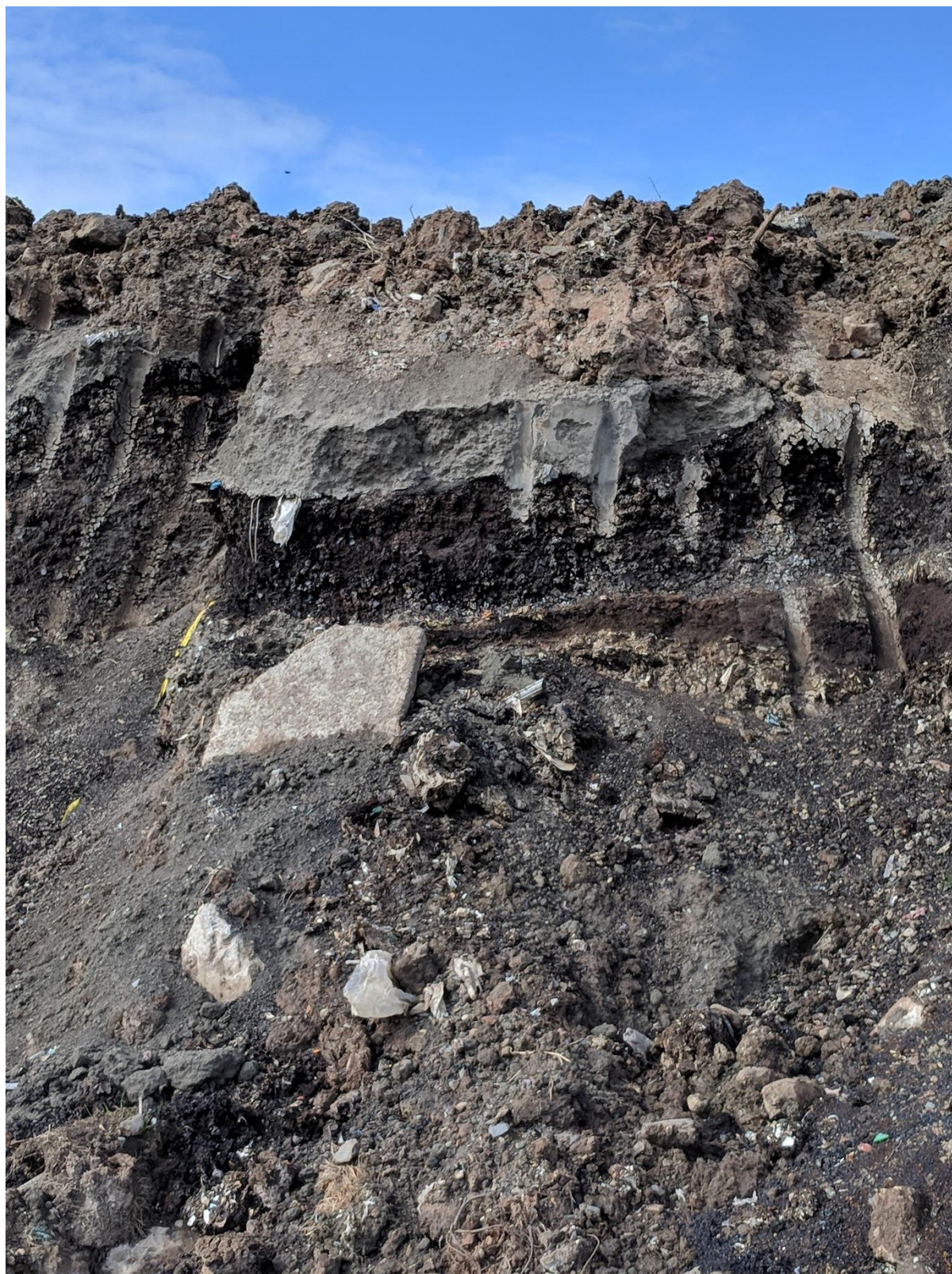
Figure 17 - Grey, black and brown bands of ash waste material exposed at surface at Tarbolton Landfill
