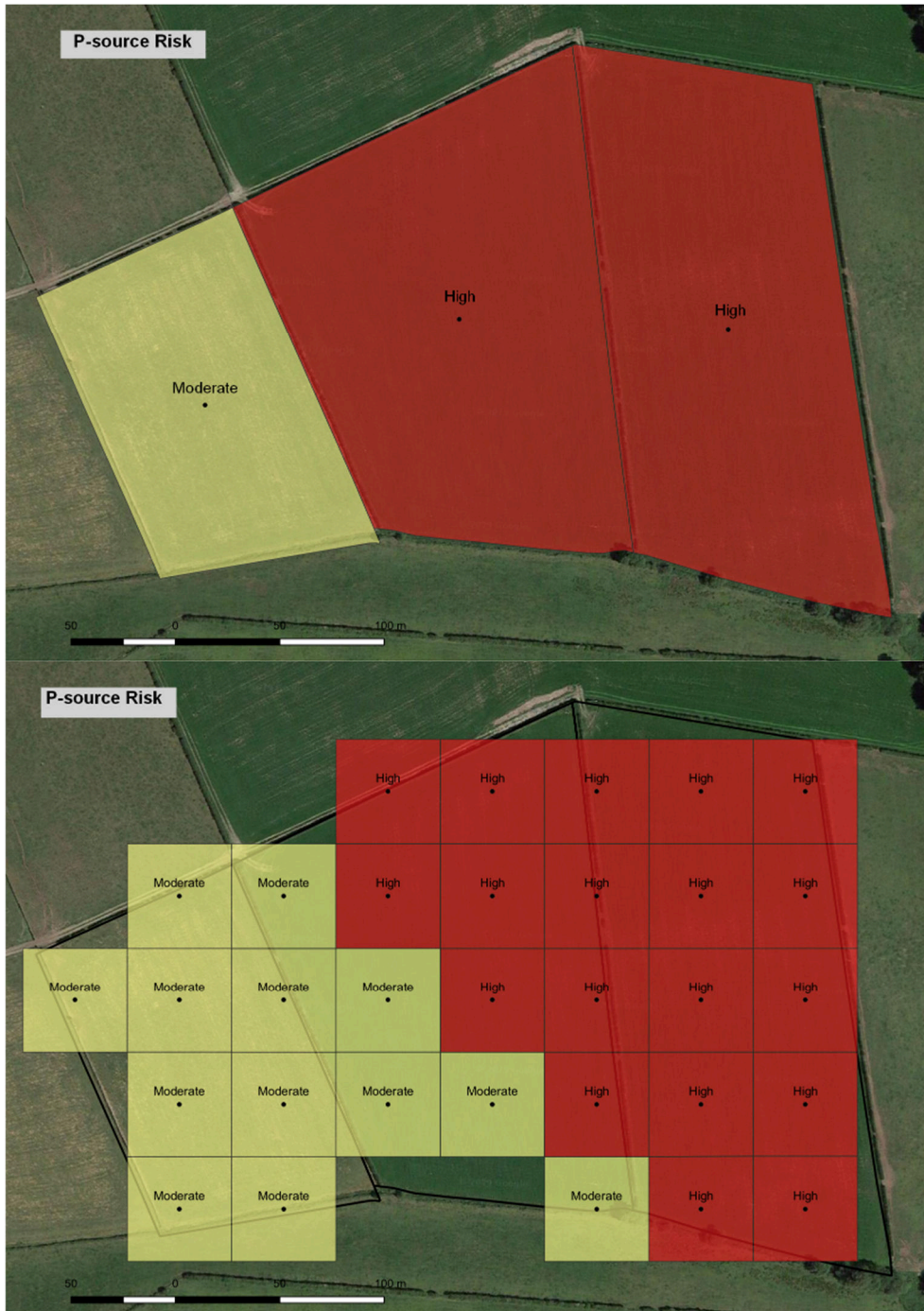
Figure 7-4. Maps of field P-source risk assessments made using the two sampling approaches. Satellite imagery from Google Maps.
