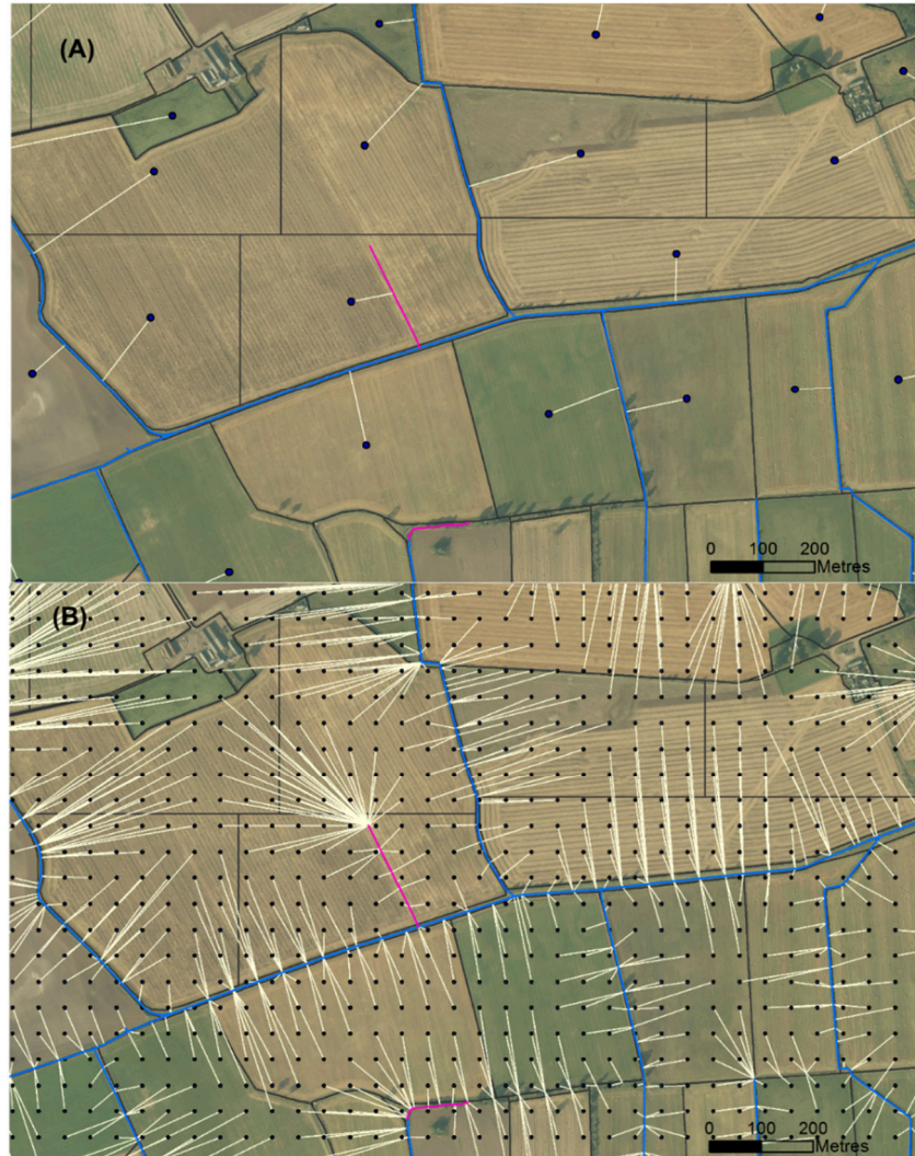
Figure 4-1. Example of mapping field connectivity to the nearest watercourse in the East Pow catchment assessed using a) samples on field centroids and b) samples based on a 50m-regular grid. Watercourse layer: blue lines represent streams/rivers and purple lines are ditches according to OS attribute table. Background satellite imagery from GetMapping PLC. © Crown copyright and database right (2019). All rights reserved. The James Hutton Institute, Ordnance Survey Licence Number 100019294.
