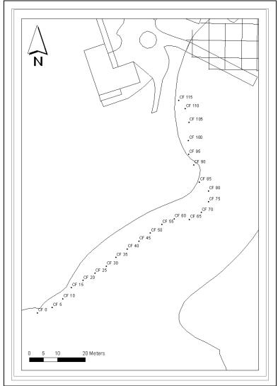
Figure 7.1 Extent of the cliff survey. Note labelling denotes (CF), Cliff face 5 metre intervals along cliff edge.
