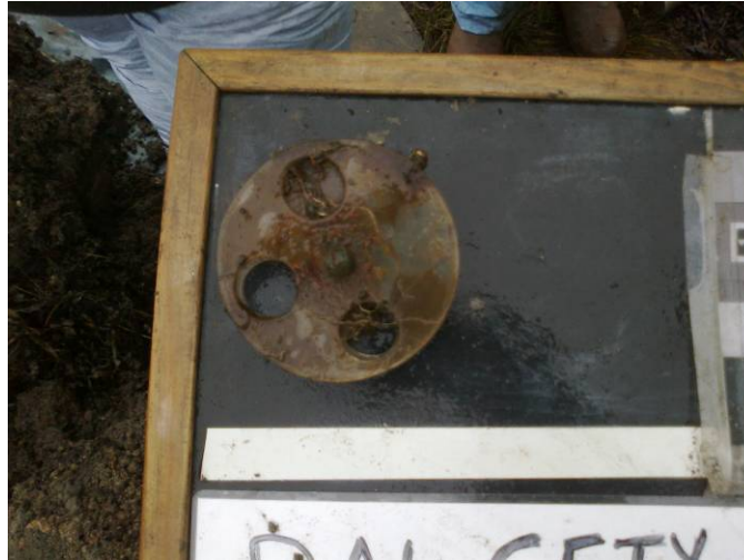
Figure 13-13: Perspex twin-layered rotating disc from TP 7/2/097 CONTAINER IN USE
