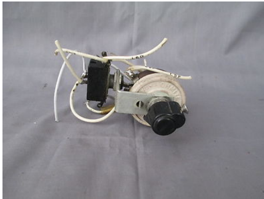
Figure 13-11: Ohmite Rheostat Switch From 1959 PA24-250 Piper Comanche
