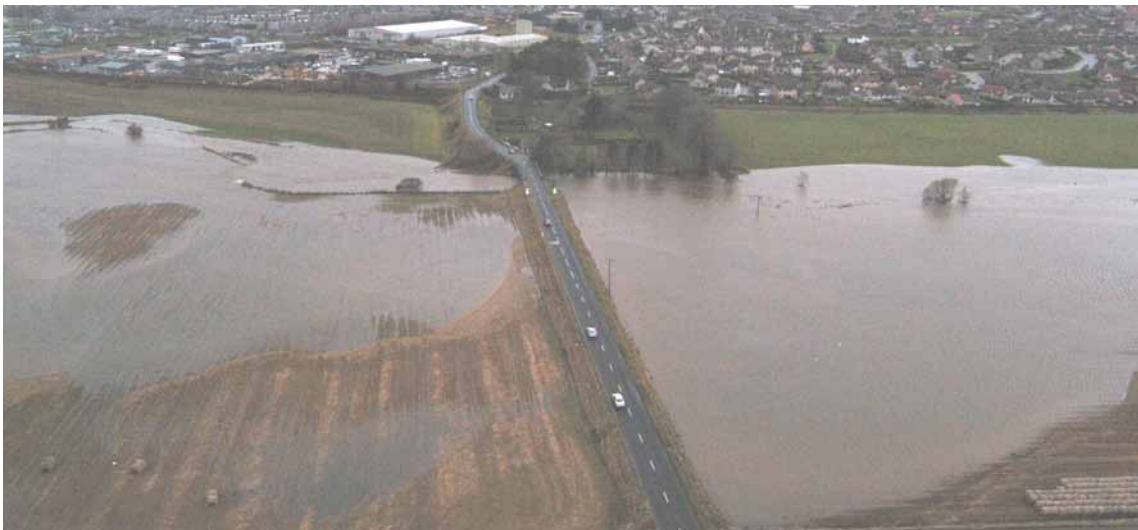
Figure 16: Crossings can constrict flood flows which can increase bank and bed erosion and alter sediment deposition, damaging river habitats and crossing structures.
