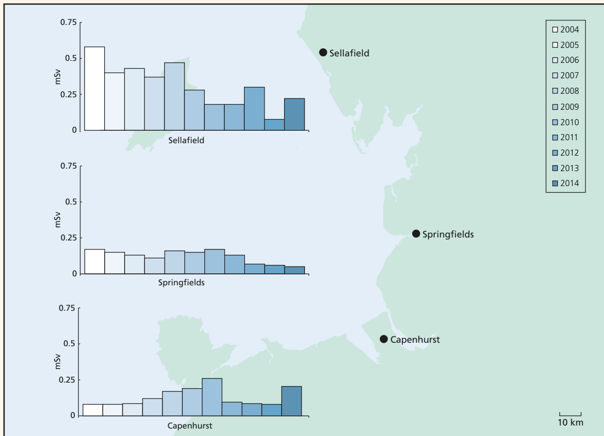
Figure 2.1. Total dose at nuclear fuel production and reprocessing sites, 2004-2014 (Exposures at Sellafeld/Whitehove/LLWR receive a significant contribution to the dose from technologically enhanced naturally occurring radionuclides from previous non-nuclear industrial operations)
