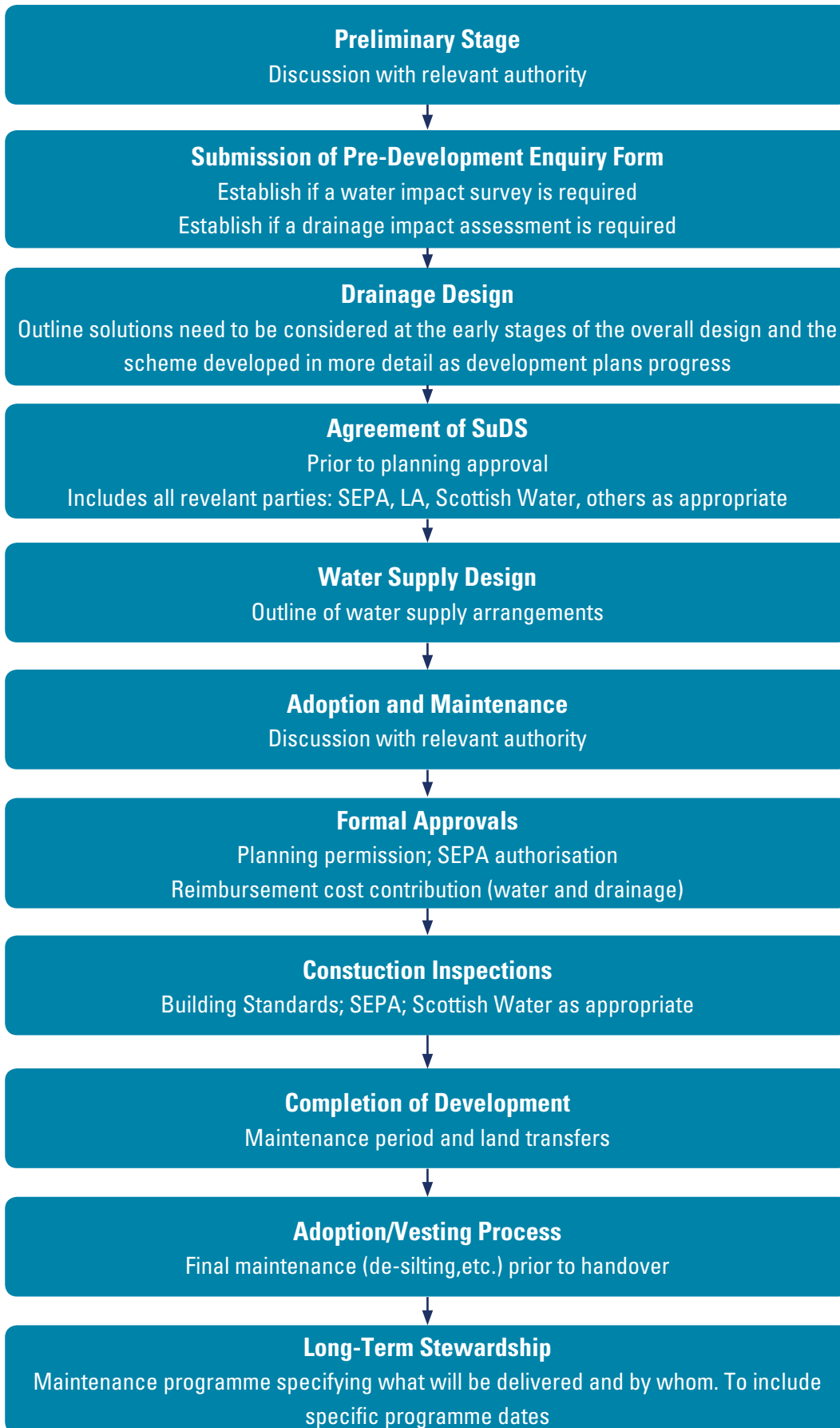
Figure 2.1 Flowchart of application and construction process
