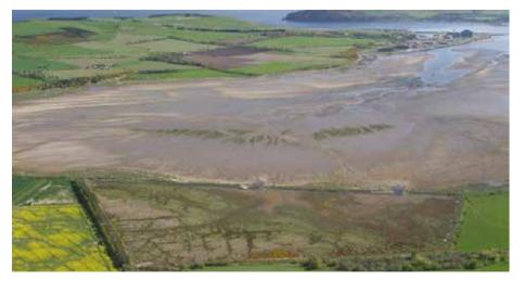
Figure 3.10. Managed realignment at Nigg Bay on the Cromarty Firth, Ross and Cromarty. Two 20m wide breaches in existing sea defences were made to allow sea water to flood a 25ha field thus reducing the maintenance requirements of the existing failing defences and creating important habiat (<sup>©</sup> N. Russell, RSPB).
