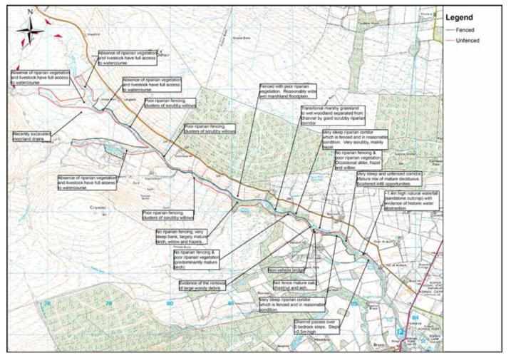
Figure 6.7. Catchment reconnaissance observations used to inform an NFM scoping study of the Allan Water, Stirlingshire (©CRESS and Halcrow).
