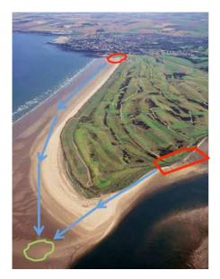
Figure 10.14. Sediment pathways at West Sands: Areas of erosion are marked in red, sediment pathways in blue and areas of accretion in green – sediment was 'borrowed' and returned to areas of erosion.
