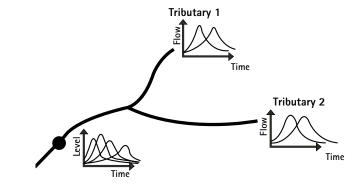
Figure 5.10. Scenario testing using a hydraulic model which has inflows at tributaries 1 and 2: In this example a series of model runs are carried out shifting design hydrographs for tributary hydrographs earlier and later in time and the impact on peak stage at a receptor further downstream is investigated. Other scenarios could involve changing the relative magnitude of the tributary hydrographs or changing the hydrograph shape.
