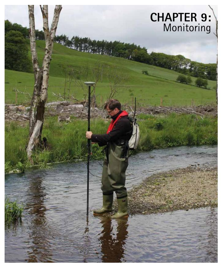
Figure 9.1. Cross section surveying on the Eddleston Water, Scottish Borders (© C. Spray).
