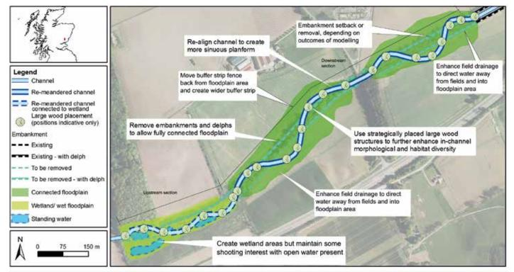
Figure 6.10. Options appraisal for restoration of a reach in the South Esk catchment, Angus (©cbec eco-engineering UK Ltd.)
