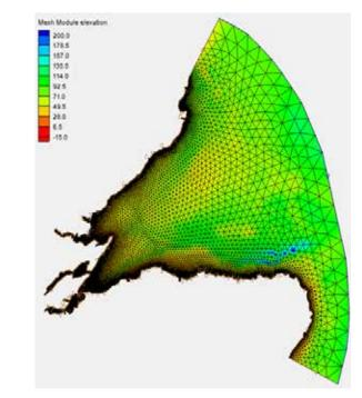
Figure 5.11. Example of a wave transformation model grid such as might be used to look at the effect of wave dissipation measures.
