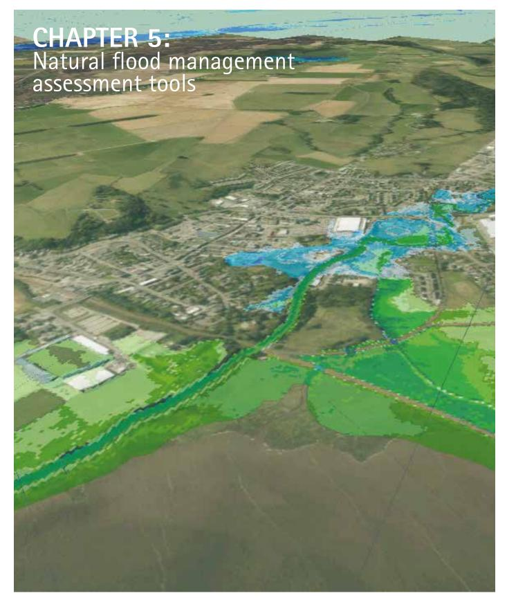
Figure 5.1. Example of a 2D hydraulic model output.
