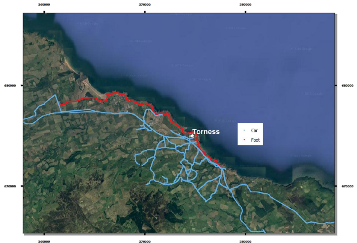
Figure A3i MoGSS coverage of Torness survey area. Red points demonstrate the area walked using the backpack system and the blue points represent roads covered by the carborne system.
