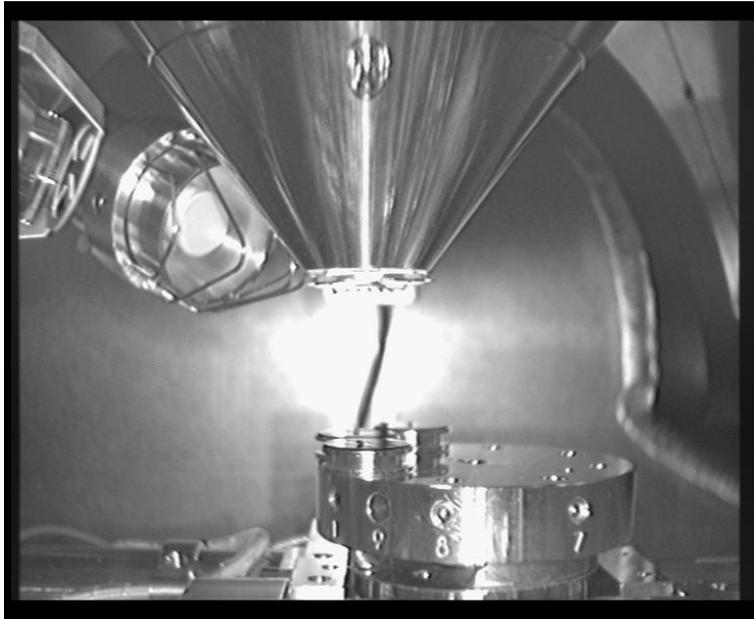
Figure 1: Infra-red camera view of three particles mounted within the SEM chamber
