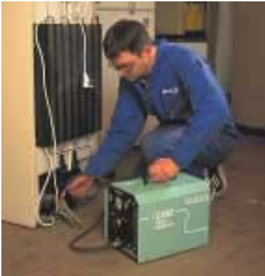
Degassing a refrigerator
