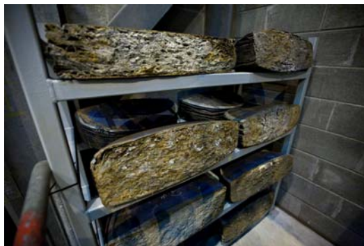
Figure 27: Compacted Pucks from Shredded Waste and Sludge Trials
