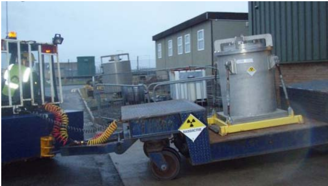
Figure 23: Spent DFR Ion Exchange Column Inside Transport Overpack
