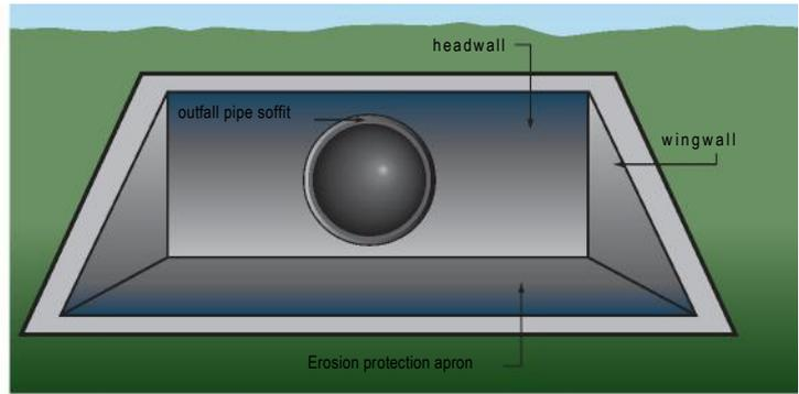
Figure 2b Typical outfall details showing the main structural components.
