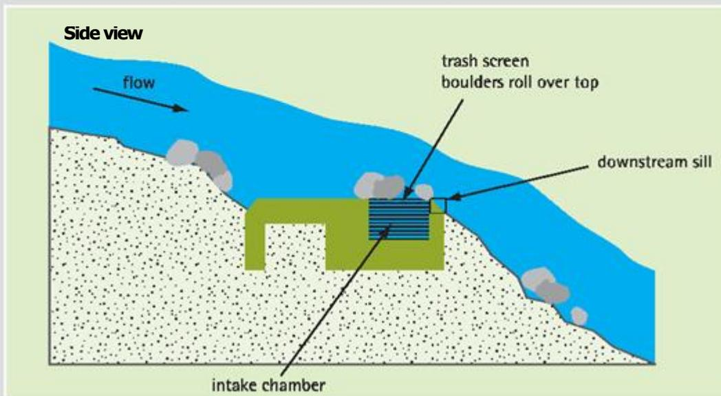
Figure 9 Schematic diagram of bed intake 'Coanda' type
