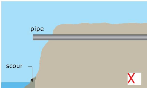
Figure 30 large height between outfall and water lead to scour
