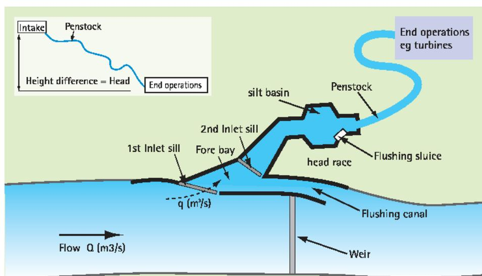
Figure 2a Schematic diagram of an intake associated with a weir showing the main structural components
