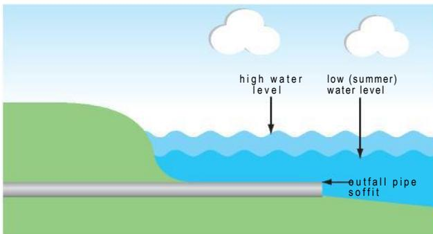
Figure 21 pipe soffit below low water levels of the loch
