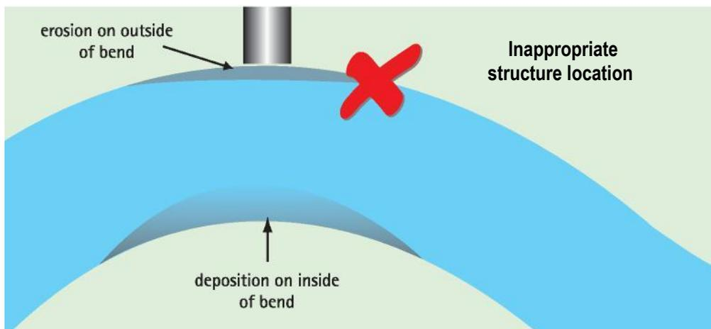
Figure 18 Incorrect structure location.
