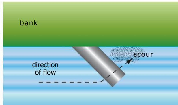
*Figure 28 and 29* Outfall pipe protruding beyond bank
