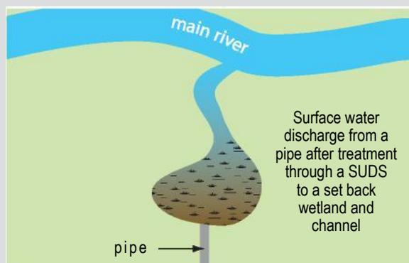
Figure 16 and 17 set back outfalls. Photograph courtesy of Robert Bray Associates
