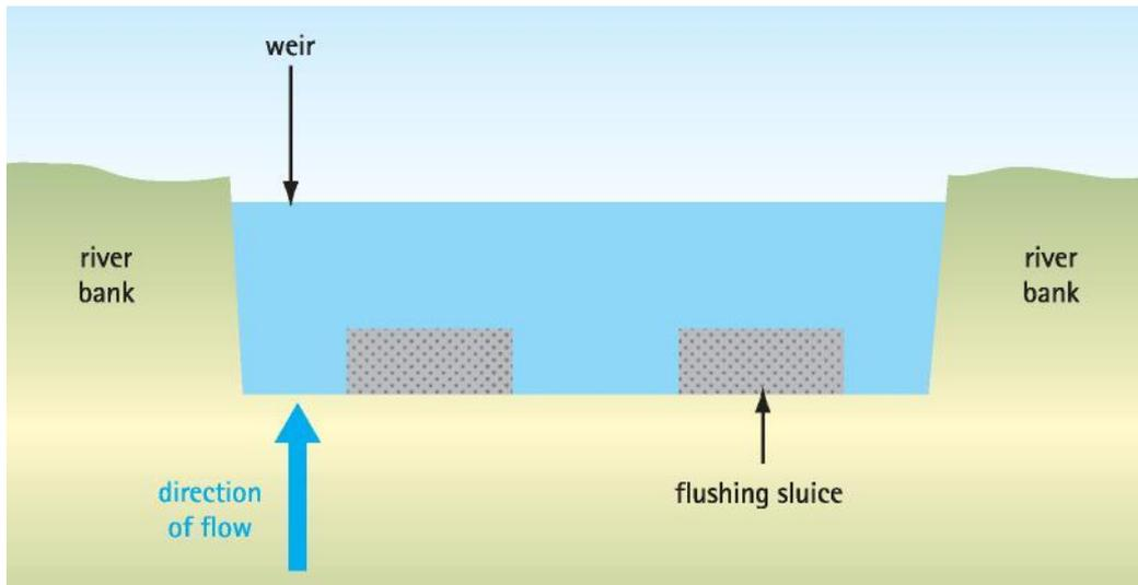
Figure 26 Schematic diagram of a weir with sluices for flushing sediment
