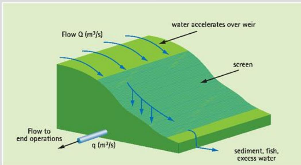
The 'Coanda' type intake (Figure 9) has a screen with a wedge wire panel installed on the sloping downstream face of a weir. This screen allows water to pass through while allowing fine sediment, larger sediment, debris and fish and excess water to flow safely downstream. Water flows through the wire mesh screen to the collection system at the base.
