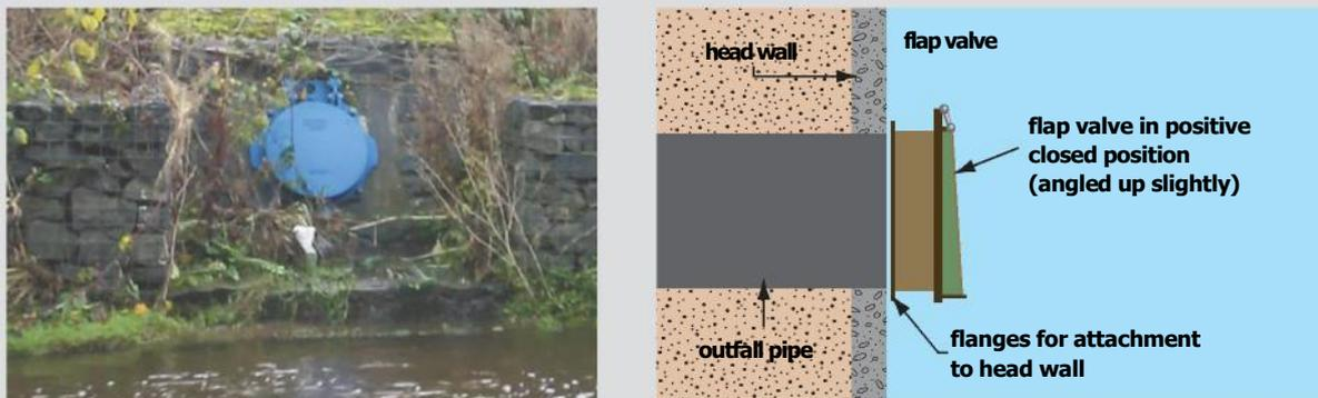
Figure 35 and 36 Outfalls with flap valve.
