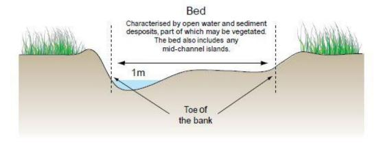
River width is the straight line distance measured between the toe of the banks of any watercourse, including any exposed bars and vegetated islands.
