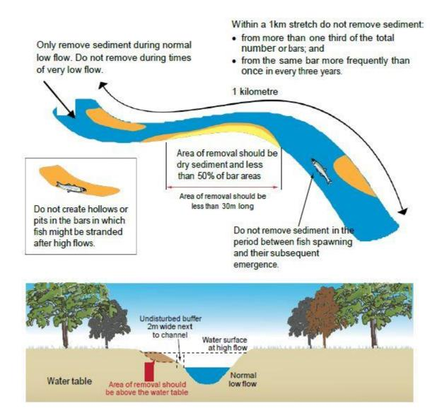
Activity L: Removal of sediment from the bed of a stretch of a river or burn that has all of the following characteristics:
