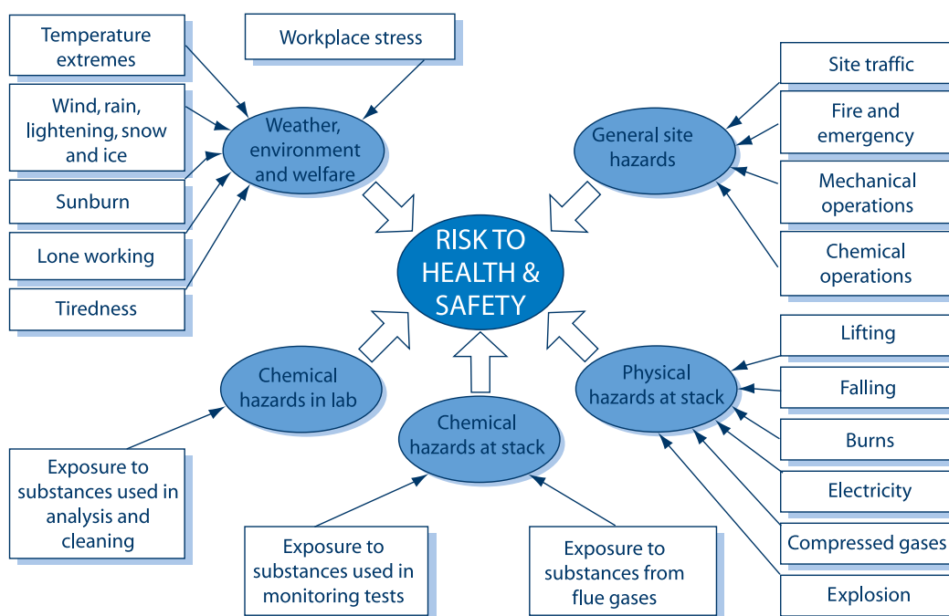
Figure 5.2 | Prominent hazards associated with stack monitoring
