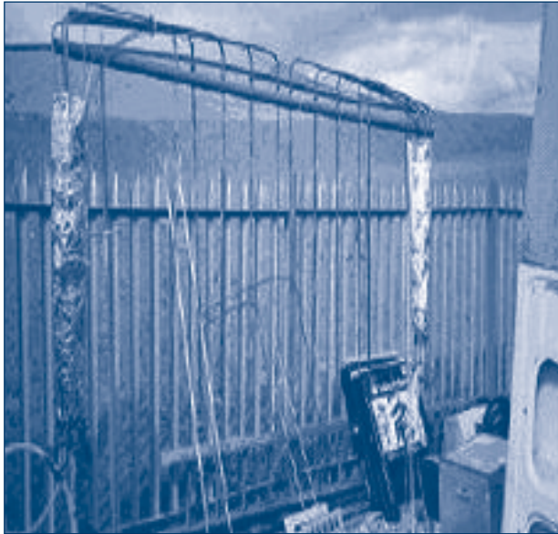
Figure 6.2 | Multiple-probe system for end-of-pipe sampling
