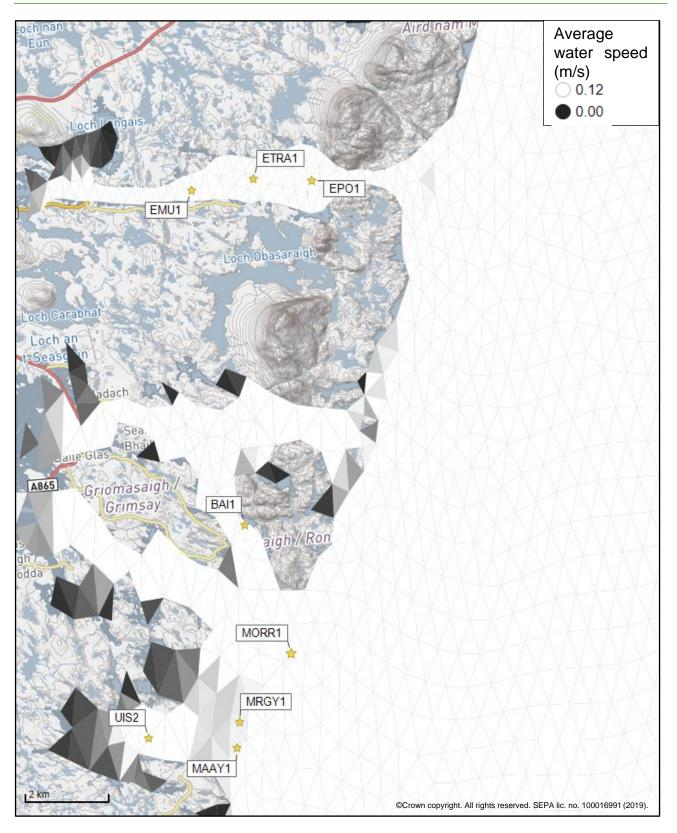
Figure 2: Modelled average water speed (metres per second – m/s) in the sea area surrounding the proposed site (Morrison's Rock (MORR1)).
