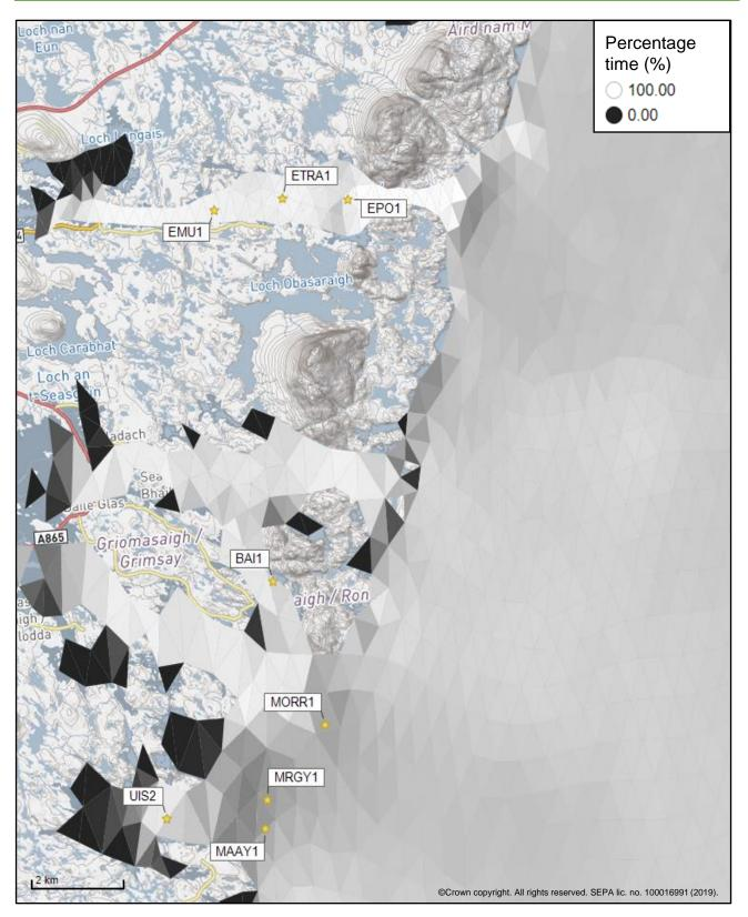
Figure 3: Modelled percentage of time the water flow speed is above 0.095 m/s in the sea area surrounding the proposed site (Morrison's Rock (MORR1)).
