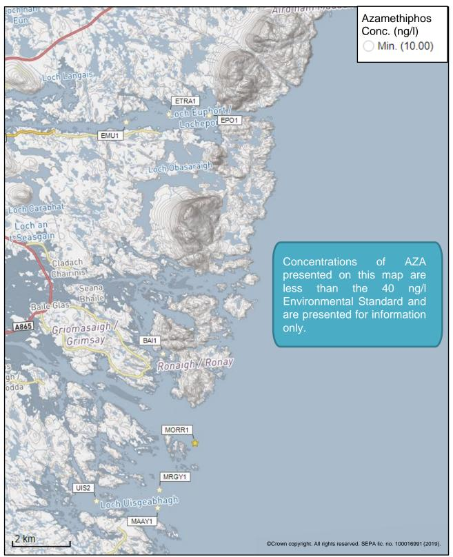
Figure 6: Modelled average Azamethiphos concentration over four days from neap tide release for the proposed site only (Morrison's Rock (MORR1)).
