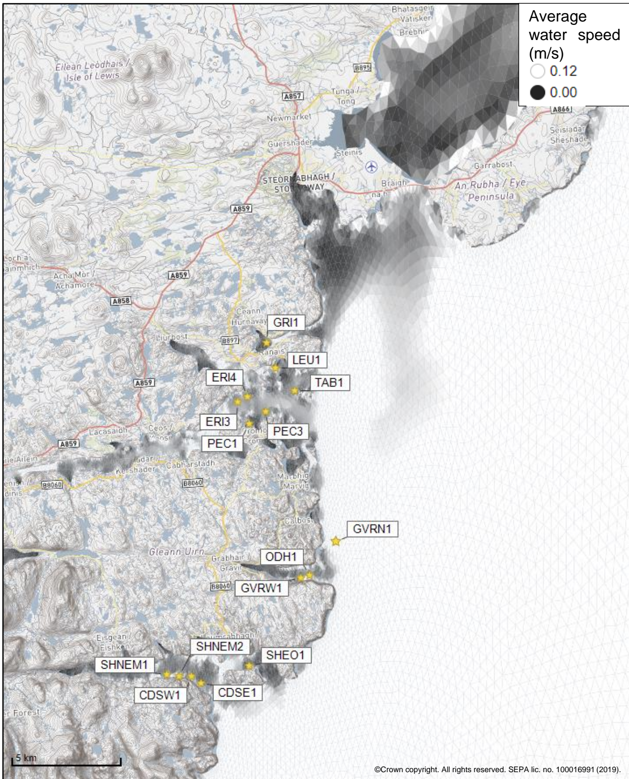
Figure 2: Modelled average water speed (metres per second – m/s) in the sea area surrounding the proposed site (Gravir North (GVRN1)).
