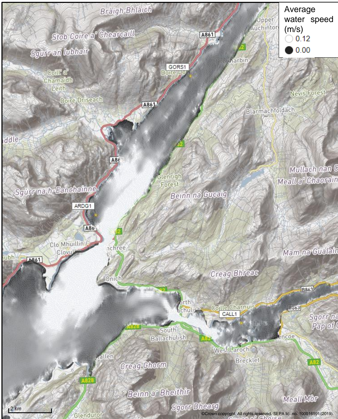
Figure 2: Modelled average water speed (metres per second – m/s) in the sea area surrounding the proposed site (Ardgour (ARDG1)).
