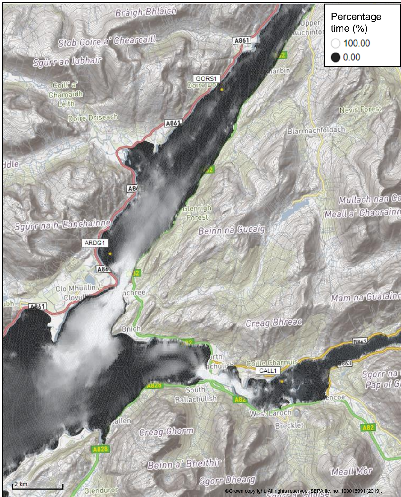
Figure 3: Modelled percentage of time the water flow speed is above 0.095 m/s in the sea area surrounding the proposed site (Ardour (ARDG1)).
