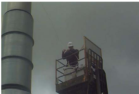
Figure 3.1: Sampling a point source
