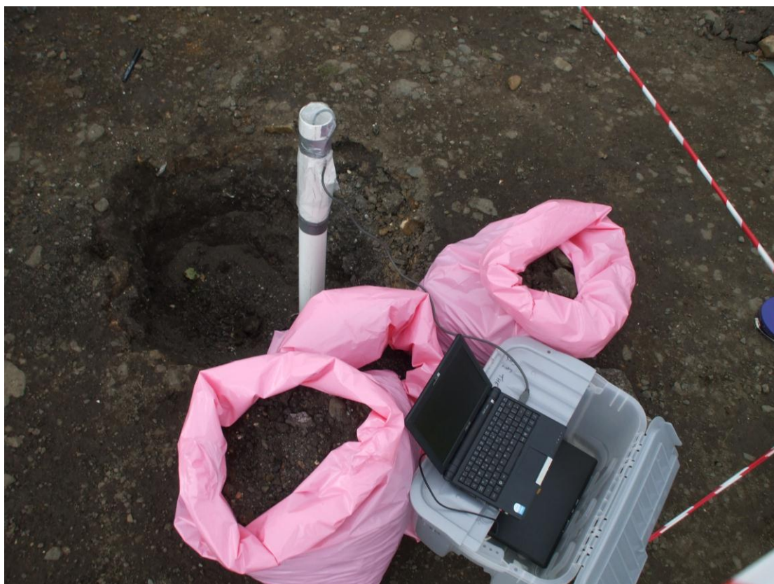
Figure 8. Deployment of the 50 mm x 50 mm NaI(Tl) detector at 1.5 m depth.
