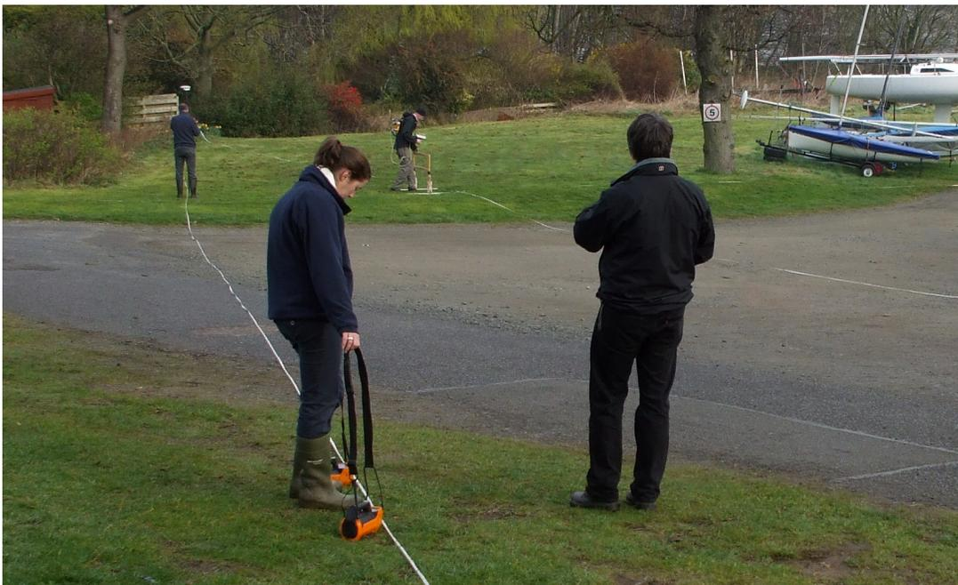
**Figure 1.** GPR, DGPS and Gross Gamma counting along predefined transect
