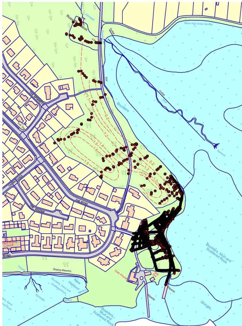
**Figure 8.** Sketch contour interpretation of the GPR data in area B
