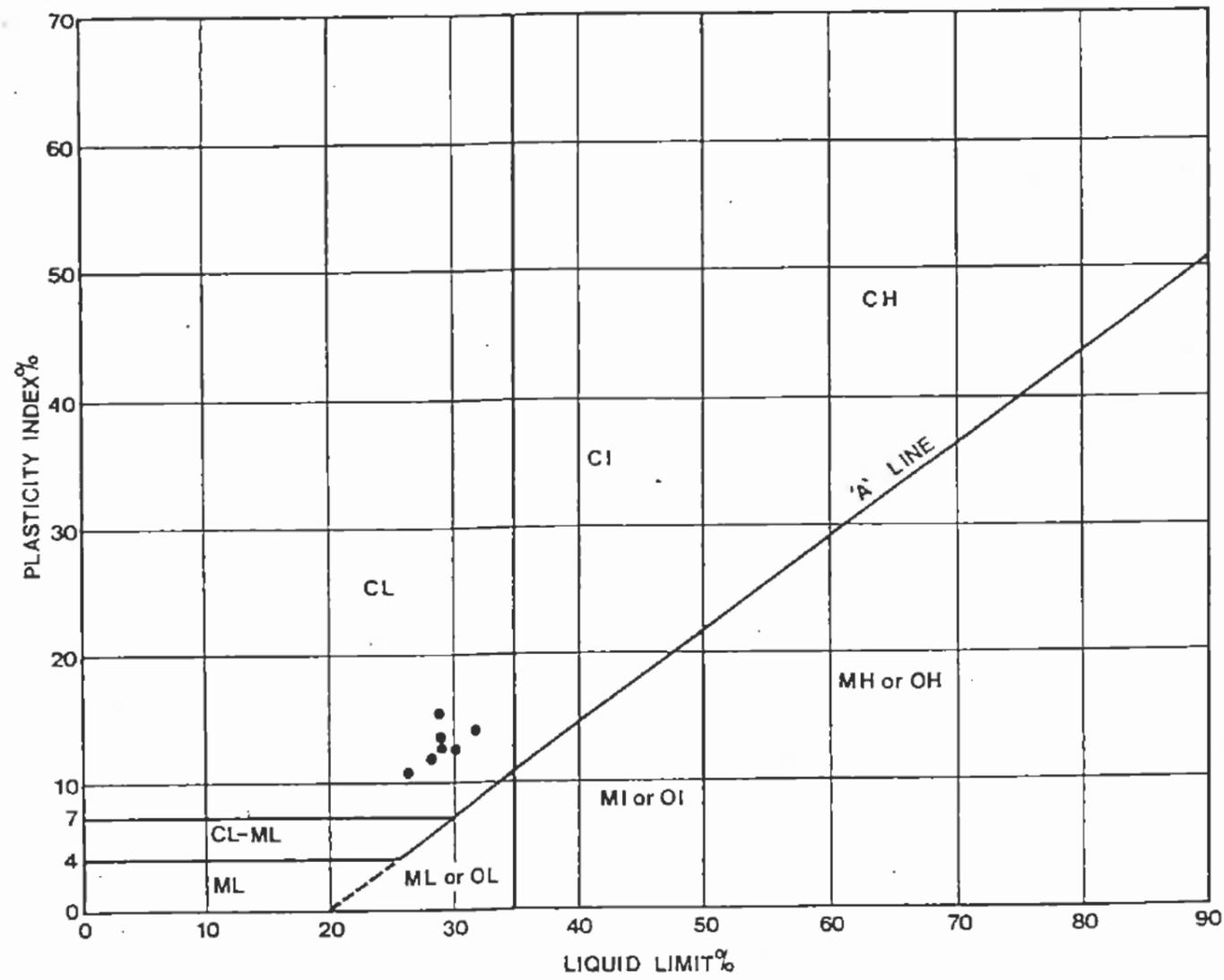
The fine grained soils are divided into three groups: inorganic silts (M), inorganic clays (C), and organic silts and clays (O). The soils are further divided into those having liquid limits lower than 35% (L), between 35% and 50% (I) and higher than 50% (H)
