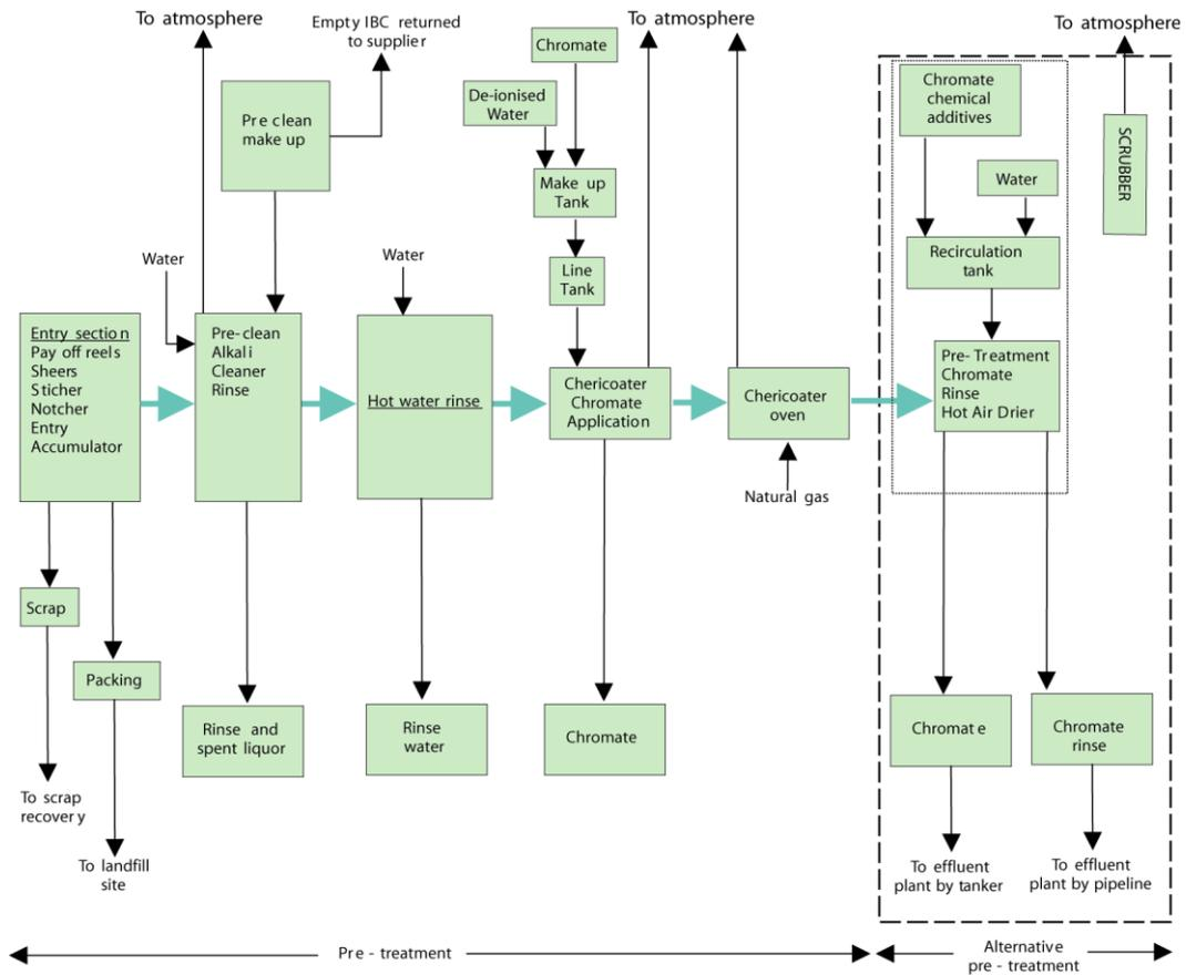
Figure 3.4 - Flow diagram of a typical rewind and colour coating line
