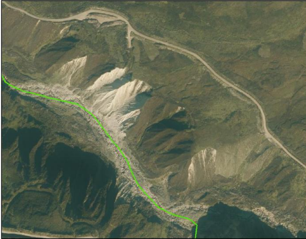
Figure 17: Aerial photograph showing gully/hillslope erosion adjacent to the high recovery potential section which is delivering high loads of sediment directly into the channel. Location within the catchment is shown on Figure 18.
