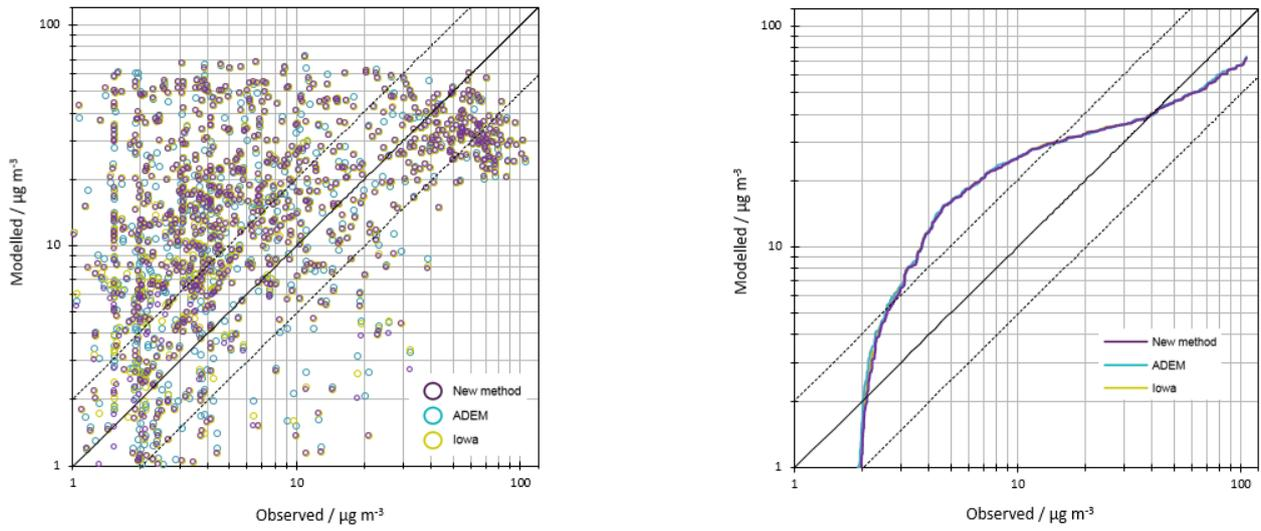
The validation exercise demonstrated little difference between each method, primarily due to combustion and process plant emissions being the dominant contributor to predicted impacts at the monitoring station. The Wood method, however, did produce mean predictions closer to those observed, with the highest correlation co-efficient and FA2 value, and lowest mean gross error and fractional bias values.
