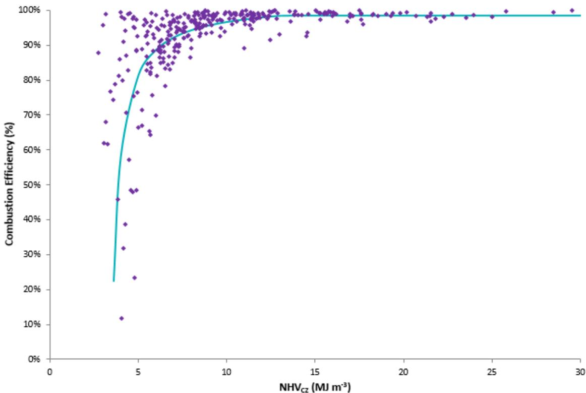
Using the US EPA (2012) data, Wood has developed a relationship linking the combustion efficiency to the net heating value of the mixture in the combustion zone. The relationship is provided below and plotted graphically on Figure A.1 as the solid light blue line.
